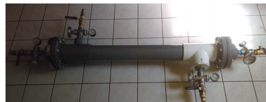
S&T Chiller Heat Transfer Area: 10.97 ft 2
